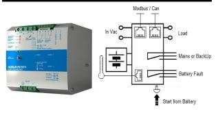
Input: Single-phase 115 - 230 - 277 Vac Output Selectable Load:12 Vdc 15A; 24 Vdc 10A Output Battery charging: 12 Vdc 15A; 24 Vdc 10A Suited for the following battery types: Open Lead Acid, Sealed Lead Acid, lead Gel and Ni-Cd Automatic diagnostic of battery status, Battery Life Test function (internal Battery Impedance) Charging curve IUoU, constant voltage and current Four charging levels: Boost, Absorption, Trickle, Recovery
